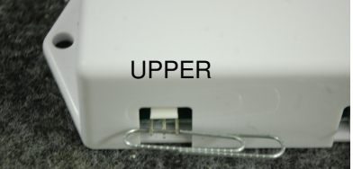
The 3 pin output can be shorted by lacing a paper clip or stiff wire alternately over and under the pins, or shorted with an alligator clip.
