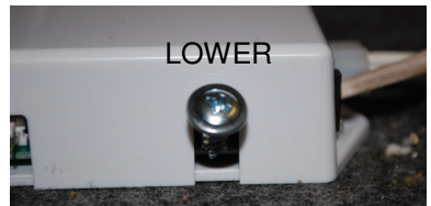
The 2 pin output can be shorted by wedging a small screw or other metallic object between the pins. Or shorting with an alligator clip.
